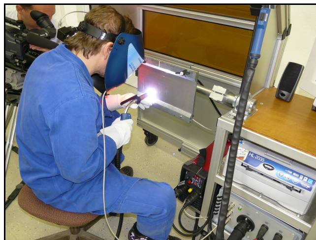
Figure 2: Training of the welding position PF for MAG welding using "fir tree welding"
